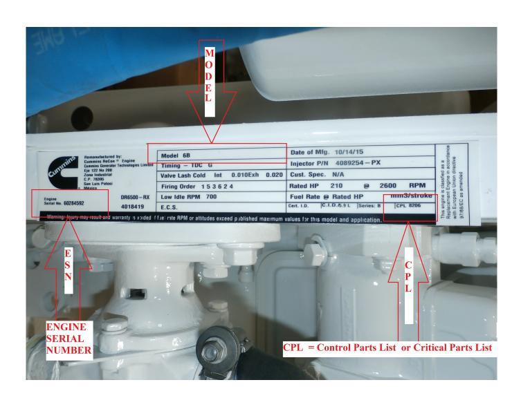
Cummins Engine Serial Number Decoder
